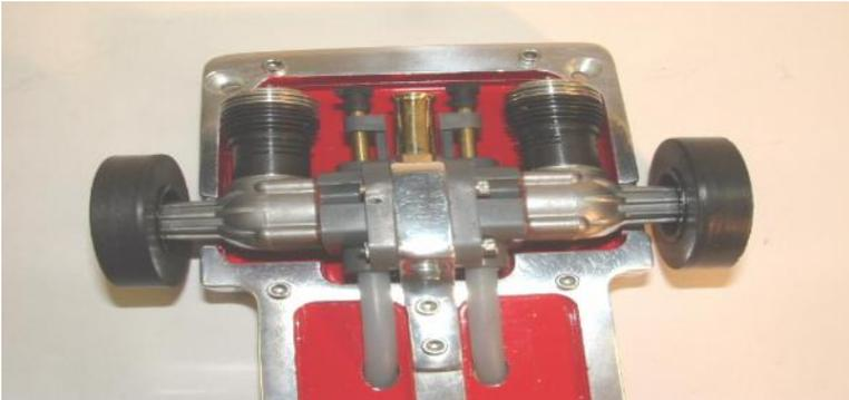
The chassis and fuel tank were of course milled from billet aluminum and on the bottom of the chassis I milled it out to look like a drive train, painting the milled out area red to match the roll cage. I extended the fuel and vent line to protrude through the front air dam to help pressurize the system and to make fueling easier.
